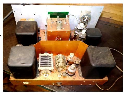
ship was done by someone who knew what he was doing and looked very professionally done. Although no measurements were made on the resistors, the HV filter capacitors were checked for shorts before applying power and appeared to be good.
