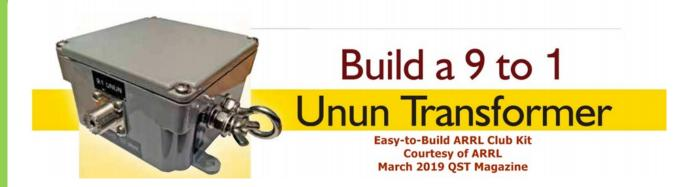
At long last, the arrangements for the assembly of the BVARA's 9-1 Unun kits have been finalized. Two 'Betas' have been assembled and tested. Both tested well, below 1.16 to 1 or lower on all bands into a 450-ohm load. The performance looks very promising for field use.
