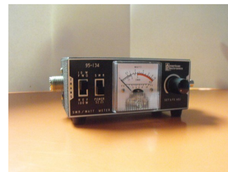
American Electronics SWR/Watt Meter, model 95/134. 52 Ohms, 100 W $20.00 plus S&H.
